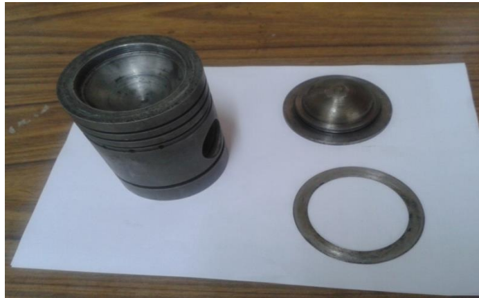
Fig.1 Photographic view of insulated piston
