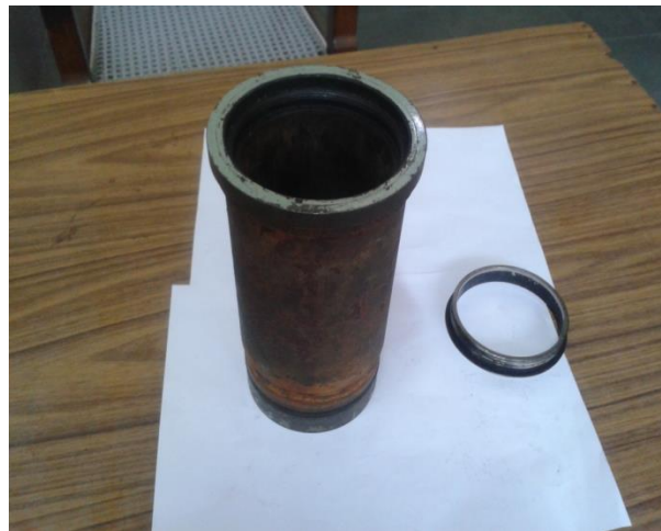
Fig.2. Photographic view of insulated liner
